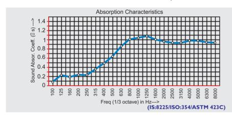
Product Characteristics Accosound is a blended elastomeric nitrile rubber acoustic absorber having open cell structure with complex pore geometry for effective absorption of air-borne sound across a broad range of frequencies.
