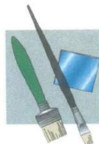
BRUSHES (VARIOUS) AND FLEXIBLE SPATULA for spreading glue and painting.
